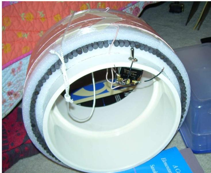
In order to lower the FSL into the enclosure, the FSL must be first partially lowered in to clear the variable capacitors. Once the capacitors and the switch are close enough together, the connections can be made, and the FSL can be lowered all the way in. This can be tricky – you might want to have someone holding onto the FSL while you make the connections!
