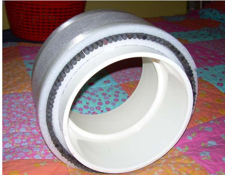
Next, I would the Litz wire in "contra" orientation, leaving about 1/4" between the two coils. After the coils were wound, and secured with adhesive tape, I threaded the four wire end through the ferrite sleeve and into the center of the PVC coupler, in order that they could be secured to the band switch.
