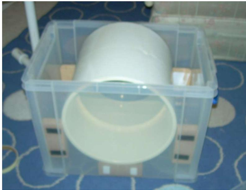
The next step was to wrap one layer of half-inch thick foam around the coupler, providing a foundation for the ferrites. Note that the foam stops about one inch from the edges of the PVC coupler in order to provide a place for the supporting blocks to contact the PVC coupler.
